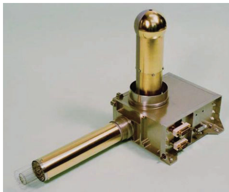
Figure 11: COmetary Pressure Sensor (COPS). Image credit: Balsiger et al. (2007)
