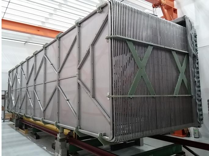
Figure 3.4.: The field-cage of MicroBooNE with direct view on the back-side of the cathode plane. The anode plane is realized using three layers of wires which can be read-out [5].
