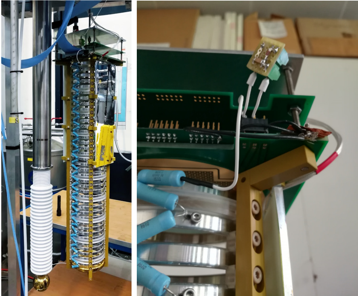
Figure 5.1: The prototype VIPER TPC at LHEP , University of Bern. Left: VIPER and two 10\text{ cm} \times 30\text{ cm} \times 0.4\text{ cm} ArCLight modules with mirrors on their back plane, mounted vertically on top of the TPC . The blue resistor chain connects the cathode and the anode via the aluminium field cage rings. The HV feedthrough with its white ceramic insulator is visible next to the TPC . Right: A close-up picture of the top of VIPER shows parts of the golden pixel plane mounted at the end of the TPC drift volume. A dummy PCB directly above the pixel PCB is intended to protect the wire bonded ASICs of VIPER . Also visible is a part of one ArCLight module, facing with its TPB coated side towards the active TPC volume.
