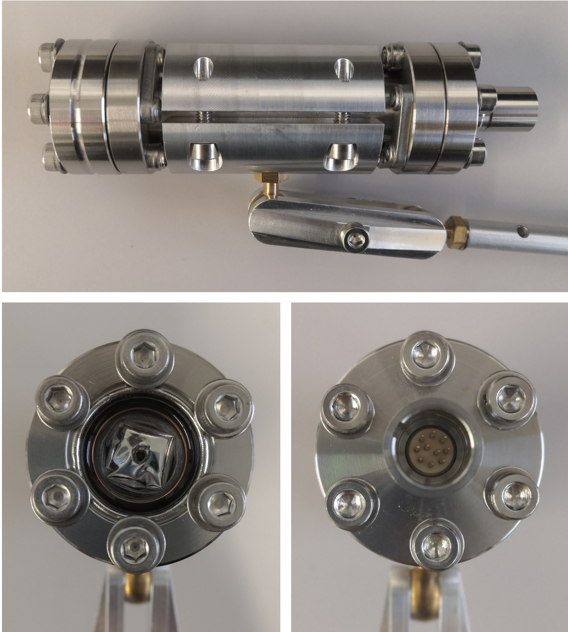
Figure 5.30: Cryocamera designed for use in LAr . Top: The camera is housed in a stainless steel tube with a length of \approx 7 cm with standard CF-16 flanges welded at the end caps. Bottom left: Front view of the cryocamera, with a CF-16 borosilicate window. Bottom right: Rear view of the cryocamera, showing the CF-16 10-pin feedthrough.
