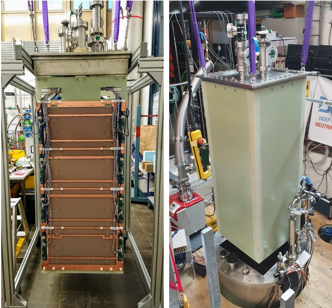
Figure 5.19: Fully assembled Module-0 and insertion into the LAr cryostat. Left: The Module-0 is bolted on the vacuum insulated stainless steel pillow of the top flange, supported by an aluminium frame. Right: The Module-0 detector, inserted into the G-10 sleeve to enable an improved LAr recirculation, is ready to be placed in the LAr cryostat.
