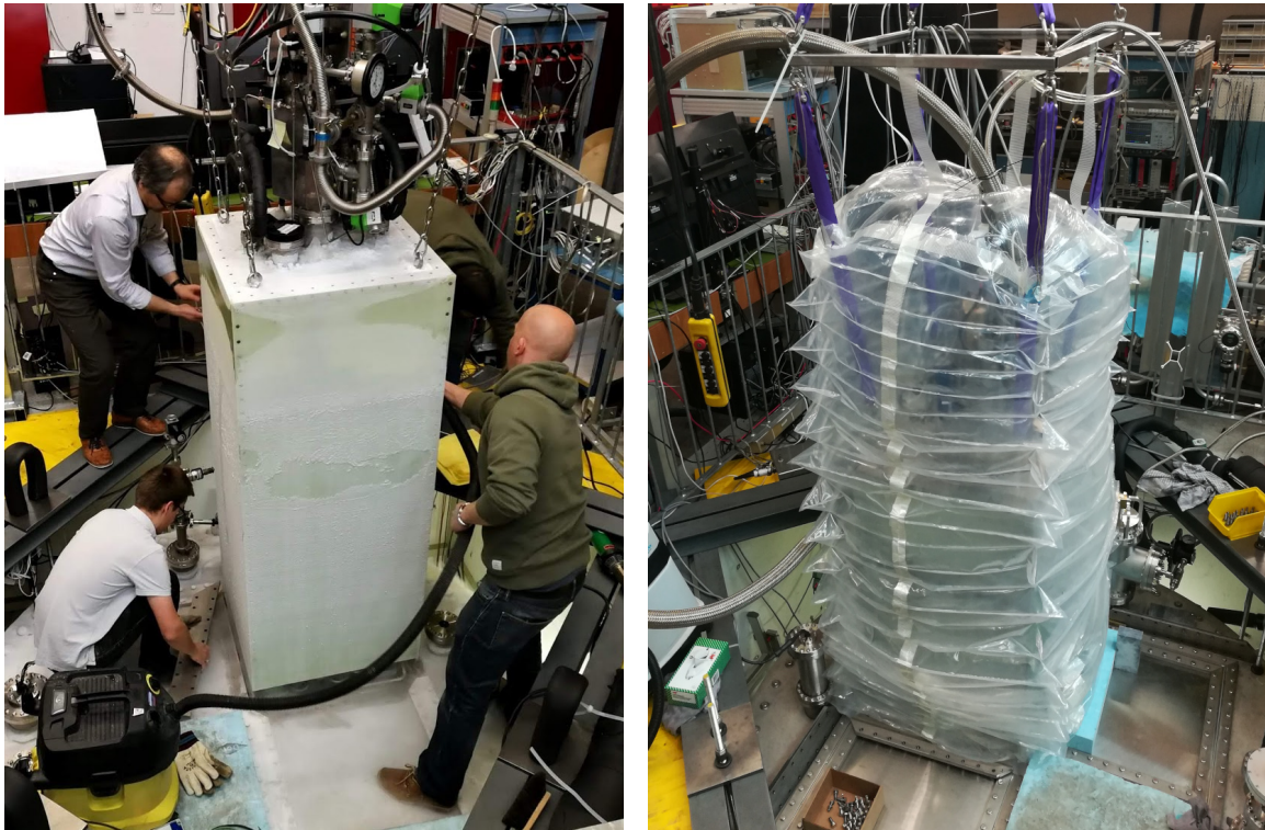
Figure 5: Cold extraction of an early module prototype from the cryostat of the ArgonCube 2x2 Demonstrator filled with LAr . Left: One attempt to extract the module from the cryostat has made use of a large flow of GAr from the inner volume of the cryostat to reduce air entering the vessel. Right: Another attempt made use of a plastic cover flushed with GAr to encapsulate the module and the cryostat opening from the surrounding atmosphere.
