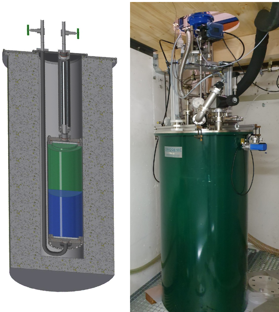
Figure 5.12: LAr filtration system as designed for the ArgonCube 2x2 Demonstrator and used in the SingleCube and Module-0 experiments. The LAr filter is immersed in a pressurised ( \approx 2.4 bar) LN 2 cryostat to provide not only purification but also LAr cooling. Left: A schematic view of the filter shows the two filter materials, a molecular sieve (blue) and a copper catalyst (green). A 5\ \mu\text{m} GKN cartridge (black) at the filter outlet is used as a particulate filter. Right: A picture showing the green vacuum insulated LN 2 cryostat hosting the LAr filter inside. A custom made liquid level-meter, as well as pressure and temperature sensors, are used to drive two PID (proportional–integral–derivative) controlled LN 2 pneumatic valves (blue) to maintain a constant LN 2 level at the requested temperature.
