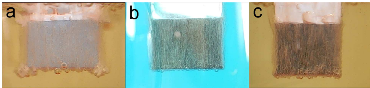
Figure S2. Optical micrographs of the electrochemical deposition by DHBT method. (a) pure-Zn, (b) pure-Cu and (c) \text{Zn}_{94}\text{Cu}_6 samples. The pictures were taken \sim 10 s after having started the galvanostatic deposition.
