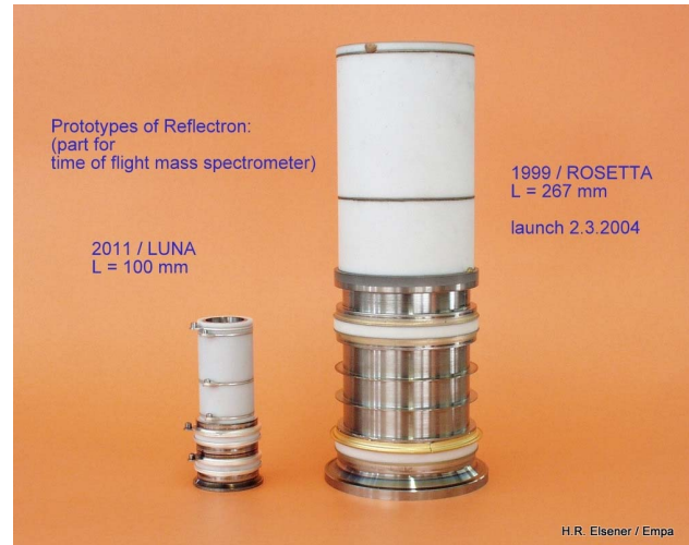
Figure 6 Integrated reflectors of previously built for Rosetta/RTOF and LUNA/NGMS (EMPA, Switzerland).
