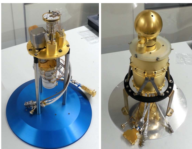
Figure 22 NIM sensor Proto-Flight Model before the start of qualification and calibration in mid-2019.
