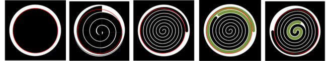
Figure 10 Different type of MCP detector anodes: circle, broad spiral, narrow spiral, and double spirals (last two). In all cases, outer anode \varnothing = 8 mm, red circle gives the active MCP area.
