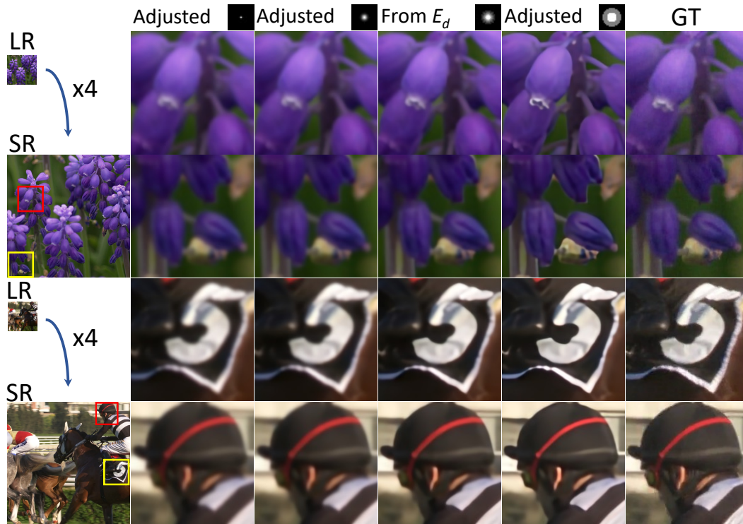
FIGURE 6.4: Degradation Manipulation. Our pipeline takes a low-resolution corrupted video from the first column and outputs the 4x super-resolved frame. Columns 2-5 show different magnified regions of the restored frame. We show the ground-truth patch in Column 6. In column 4, we have the result obtained without adjusting the latent feature from encoder E_d . Columns 2, 3, and 5 contain results obtained using latent codes from mutator model M . One can observe how blur levels vary between different columns (2-5).
