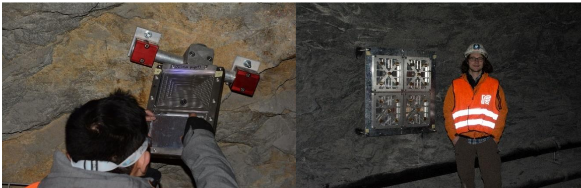
Figure 2.7: Deployed ECC detector frames in two different formats. Left: Small scale detector consisting of two ECC pouches with a total detection area of \sim 250\text{ cm}^2 . Right: Large scale detector consisting of four ECC pouches with a total detection area of \sim 1.2\text{ m}^2 . Humans are included for scale.
