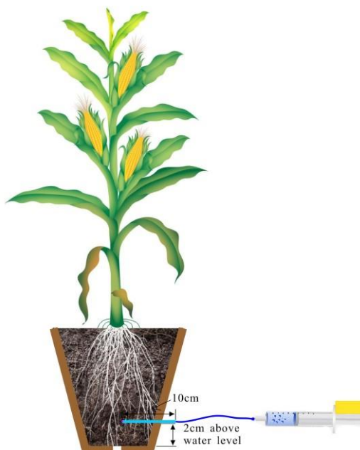
Figure S1.3. An example of a soil water sampler in a 7 L pot
