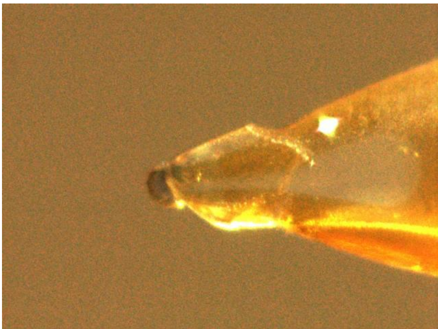
A single crystal of the compound mounted on a loop.
