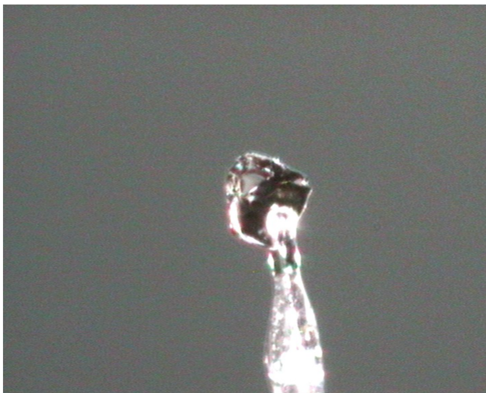
Single crystal of the compound mounted on a glass fiber.
