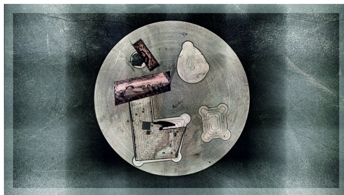
Fig. 1 – Panoramic image of the Gunflint chert thin section mounted on a steel holder (L-shaped sample, left bottom).
