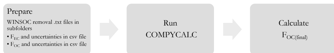
Figure S1: The workflow for corrections with COMPYCALC. The input F^{14}C values F_{EC} and F_{OC} are added as csv files to the COMPYCALC folder, the COMPYCALC script run, and with the resulting F_{EC(final)} the F_{OC(final)} value calculated.
