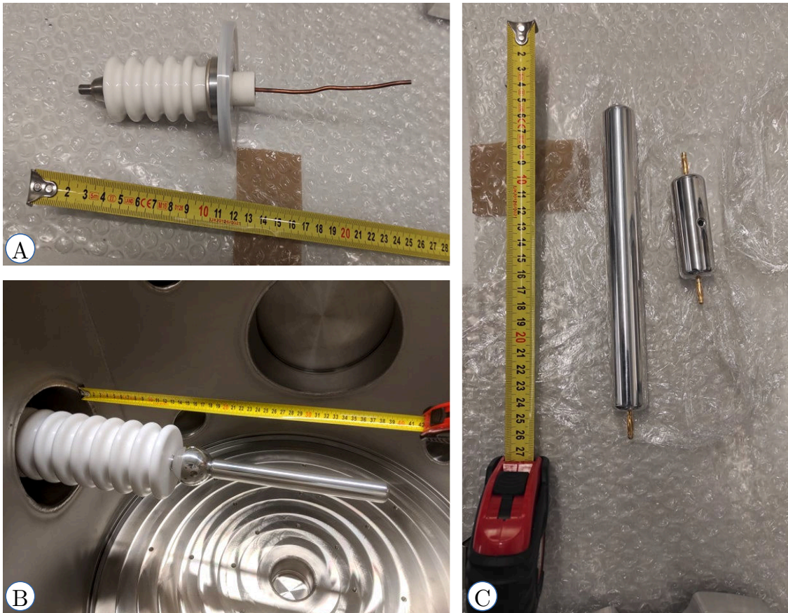
Fig. 3.14: A) Picture of the small size standard ceramic feedthrough. B) Picture of the large custom feedthrough, designed and produced in Bern for operation at \pm 200 kV. C) Examples of rods for the connection to the electrodes.
