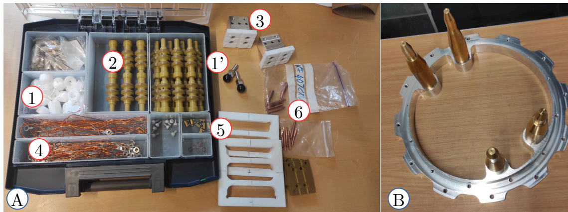
Fig. 3.13: A) Pictures of 1) Teflon heads for the alignment screws (2020), 1') alignment screws (2018), 2) insulator to hold the high voltage electrode 3) aluminum blocks to fix the ground electrodes to the rings that hold them with a Teflon piece to insulate them from it, 4) copper wires to connect the ground electrodes, 5) Teflon support to mount the electrode stack, 6) pins to connect the high voltage electrodes. B) Alignment ring with 4 pins to align the electrodes stacks with respects to the vacuum pipes. The pins matches the four holes in the rings that hold the electrodes.
