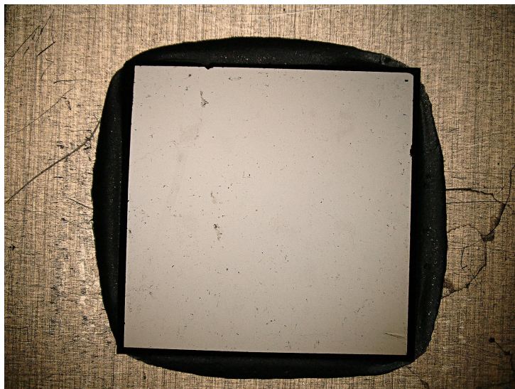
Figure 2.21.: Microscopic image of the \text{SrTiO}_3 sample glued on an aluminum carrier plate, taken after ILENA measurements at the department of chemistry and biochemistry (DCB), University of Bern. Sample: polished square with edge size 10 mm, surrounded by Ag-EP residuals (black).
