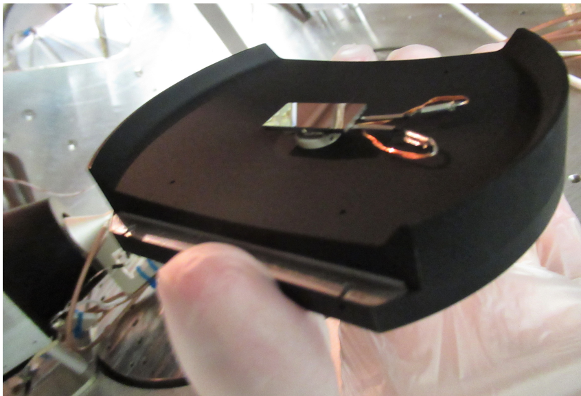
Figure 3.9.: Part of the refurbished ABM: The Acktar blackened top plate with fully assembled new tungsten plate and SS heater.
