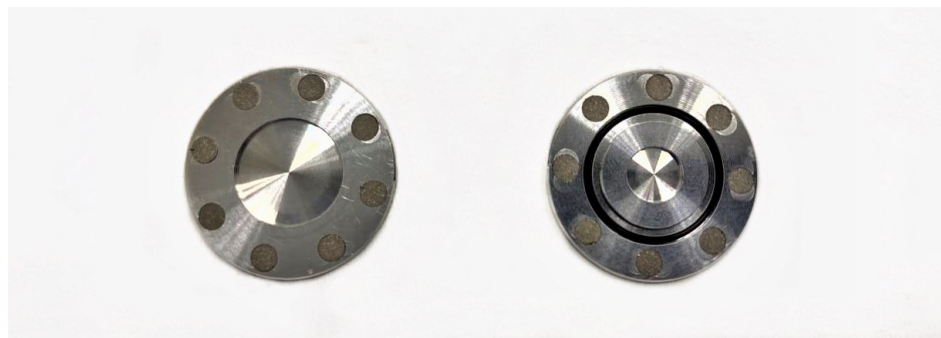
Figure 2.5: The two halves of the coin target (24 mm diameter, 2 mm thick).
