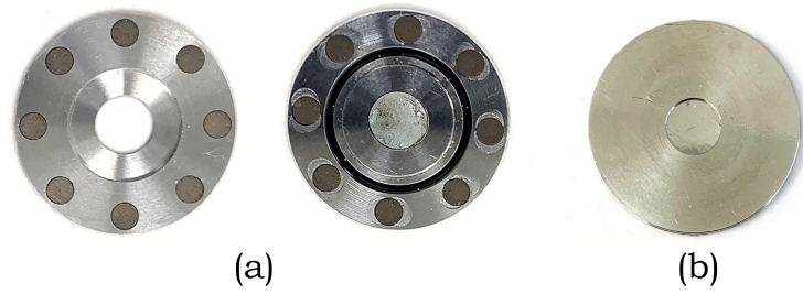
Figure 3.17: (a) Coin with a 7-mm-diameter hole in the front, containing a 6-mm enriched ^{50}\text{TiO}_2 pellet; (b) 13- \mu\text{m} -thick aluminum foil inserted in the coin to prevent the pellet leakage during the irradiation.
