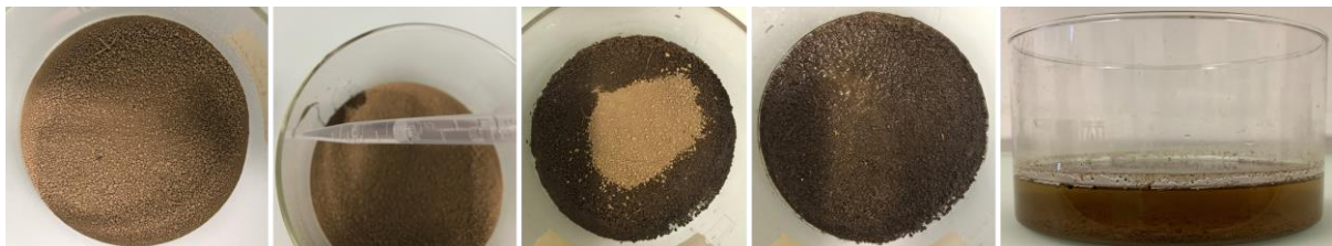
Figure S1.4: Fractionation steps for adding density solution to the soil sample
