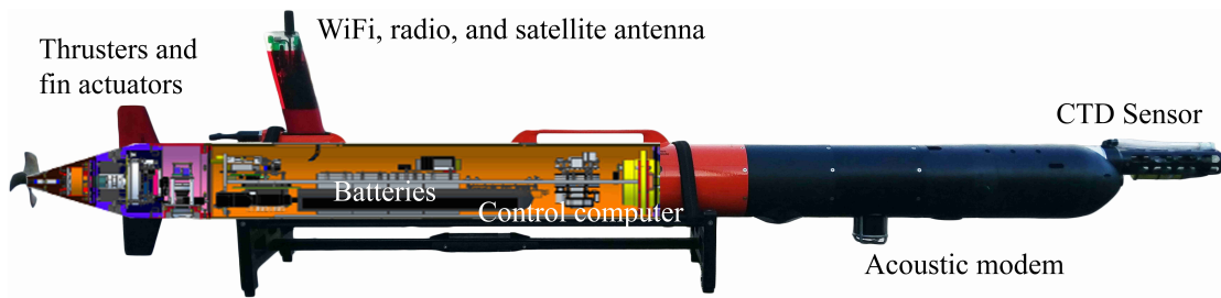
Figure 6.5: The commercially available Light Autonomous Underwater Vehicle (LAUV) platform for upper water-column exploration used in our experiments.
