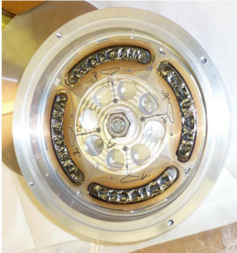
Figure 9: A rotating ^{249}\text{Cf} target wheel after bombardment with ^{50}\text{Ti} heavy ion beam. The once smooth banana-shaped target sections have suffered deformation due to prolonged irradiation. Image from [86].
