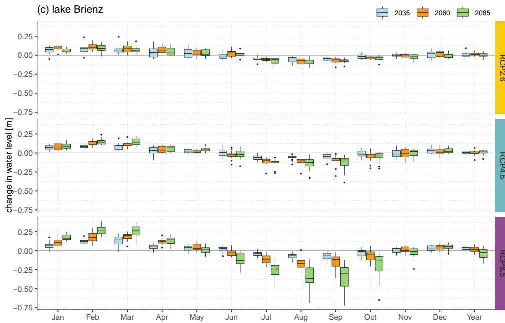
SI FIGURE 9.15: Simulated changes in monthly and annual mean lake water levels of Lake Brienz, divided into the three future scenarios (2035, 2060, 2085) and three emission scenarios (RCP2.6, RCP4.5, RCP8.5).
