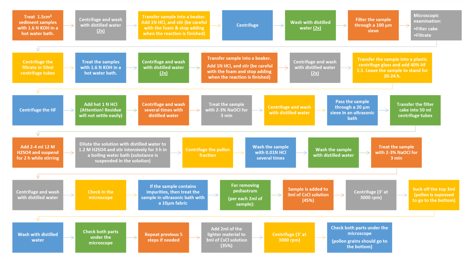
Figure 4. Lab methodology for extracting pollen concentrates. Adapted from Brown (1994).
