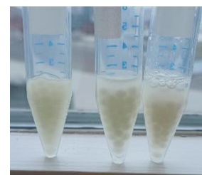
Figure 6.6: Calcium alginate beads dissolution. The illustration demonstrates how the addition of positively and negatively charged species can disrupt or weaken the ionic bonds between the carboxyl groups of alginate and \text{Ca}^{2+} ions, resulting in the dissolution of the solid matrix.
