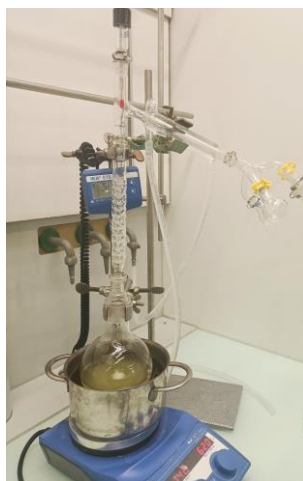
Figure 6.8: Distillation set up for the purification of isobutylamine from the SpinChem® system.
