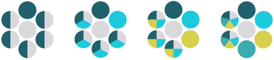
Figure 9.1. Schematic representation the seven atomic active sites as defined for the surface-activity trade-off model. From left to right the models represent the binary, ternary, quaternary, and quinary sites. The colors indicate distinct elements.
