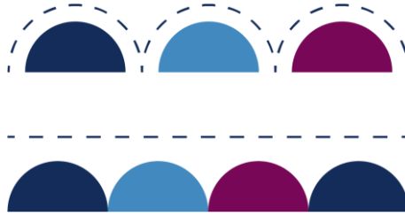
Figure 8.2. A schematic depicting the two diffusion modes of a high entropy alloy surface. Top scheme shows the individual spherical diffusion layer. Bottom scheme shows the shared planar diffusion layer.
