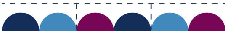
Figure 8.4. A schematic of microelectrodes composed of two active sites sharing one spherical diffusion layer, while the surface shares one combined planar diffusion layer.
