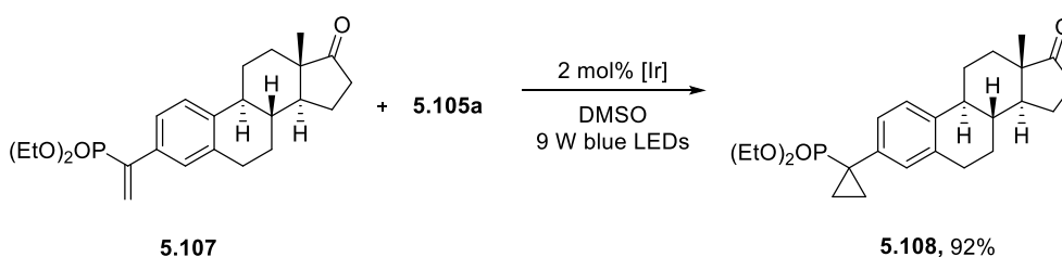
Scheme 5.36. Cyclopropanation of estrone derivative 5.107 . [Ir] = \text{Ir}[\text{dF}(\text{CF}_3)\text{ppy}]_2(\text{dtbbpy})\text{PF}_6
