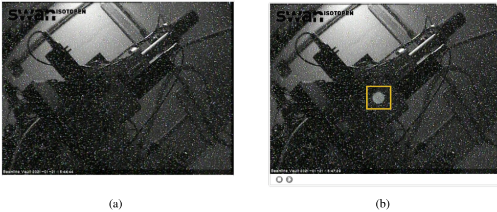
Figure 5. Image of the fused quartz sample when the beam is OFF (a) and when the beam is ON (b). The yellow square determines the ROI selected of the recorded visible light with the ImageJ software.
