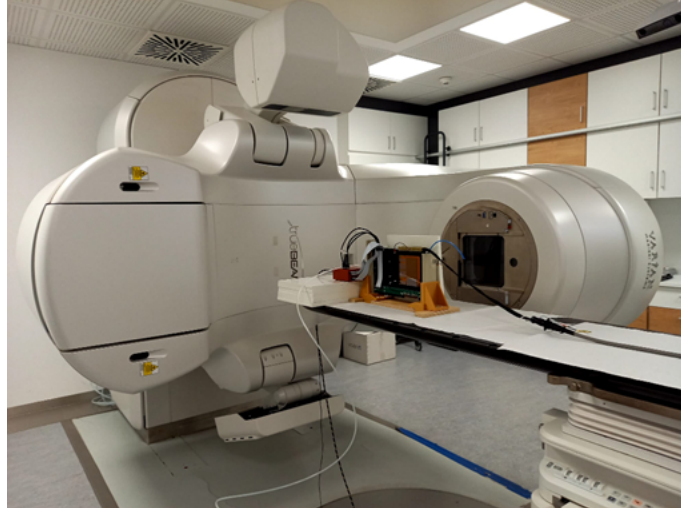
Figure 4.5: Setup utilized for conducting photon beam tests with the Varian Linac TrueBeam at Zentrum für Strahlentherapie in Freiburg. The GEM-TFT detector was situated on the treatment couch, while the treatment head was oriented at 90^\circ .
