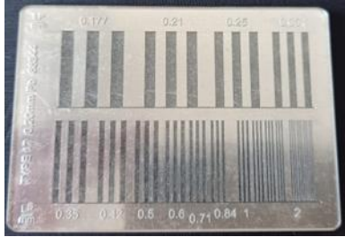
Figure 4. Line pair mask type 17 made of 0.02 mm thick lead used as an imaging target. For this particular mask, 0.5 LP/mm means that one black and one white line within 2 mm will be projected on the image sensor.
