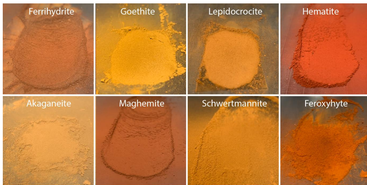
Figure 3. Ferric iron oxide powders investigated in this work using PHIRE-2. Part of each sample was compacted and then sprinkled with the remainder using very fine nylon sieves (see Methods section).
