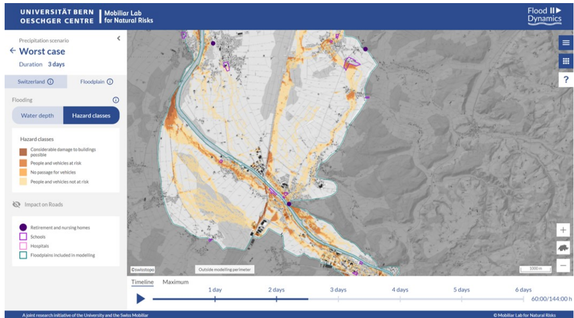
Fig. 5.1: Screenshot of the Flood Dynamics tool showing the worst-case scenario (scenario 03d-1000y_05 in 3.4) after 60 hours simulation time. The hazard classes visualized dynamically are defined in Table 3.1 and Figure 3.8 in Section 3.2.2.3.
