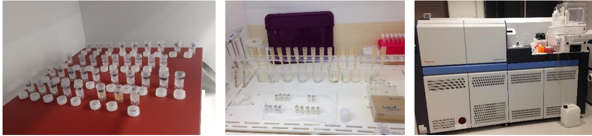
Fig. 3.15: Strontium extraction from left to right: samples drying on the hot plate; chemical extraction of strontium; MC-ICP MS in the laboratory of the Geoscience in Montpellier (pictures taken by the author during the lab work).
