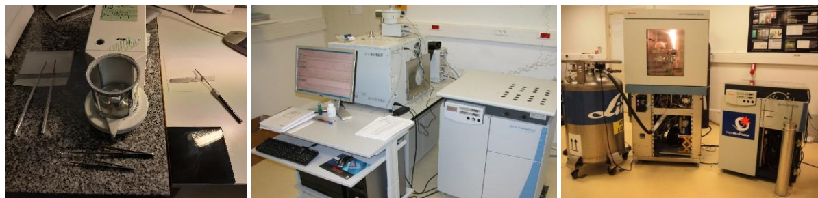
Fig. 3.17: Equipment in the Mass Spectrometry Service of the National Museum of Natural History in Paris from left to right: Mettler Toledo special accuracy weighing machine, Thermo Scientific MS DeltaV-Advantage; DeltaV-Advantage MS with Kiel IV device (pictures taken by the author during the lab work).
