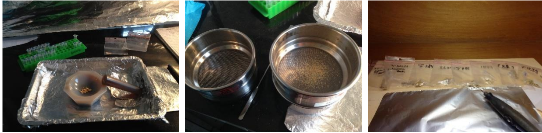
Fig. 3.12: Cleaning and leaching from left to right: cleaning and crushing of bones with mortar and pestle; fractions of bone compacta; diamond drill for taking samples (pictures taken by the author during the lab work).
