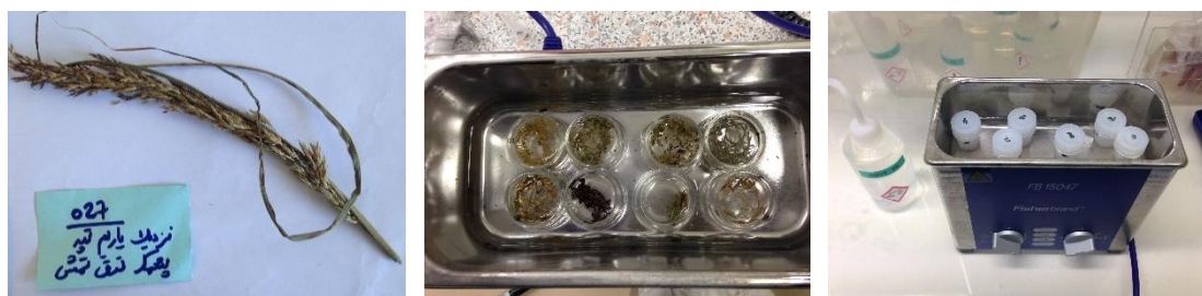
Fig. 3.14: Cleaning and leaching of dried plants for strontium from left to right: sample before preparation; dried plants rinsing with H 2 O MilliQ in the ultrasonic bath; leaching procedure of all samples in the ultrasonic bath (pictures taken by the author during the lab work).
