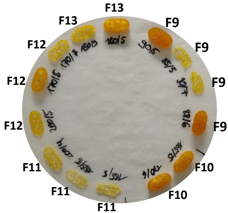
Figure A3.1: 3D-printed tablets depicted in the figure are representative of the lipid mesophase ink detailed in Table A3.2.
