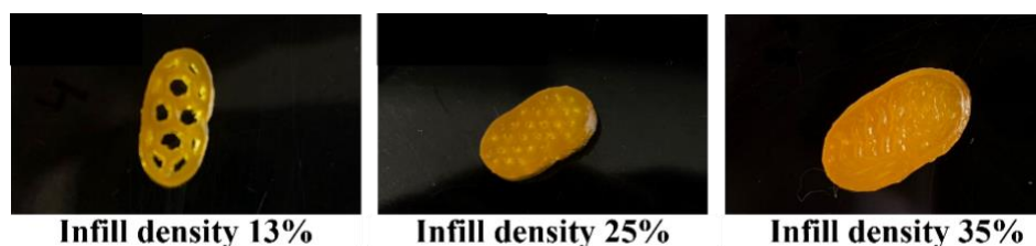
Figure 4: Samples of printlets of different infill densities.
