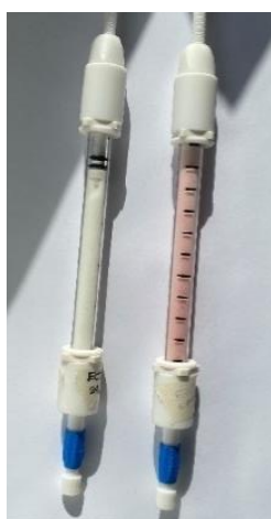
Figure 6.11 Flow column packed with immobilised EcTnaA before (left) and after (right) the experiment.
