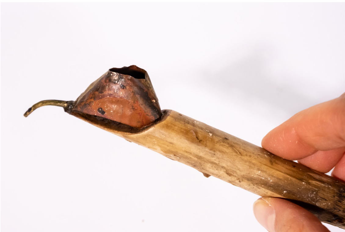
Figure B12 A canting tulis with copper tank and bamboo handle, Yogyakarta 2011. Image by the author.
