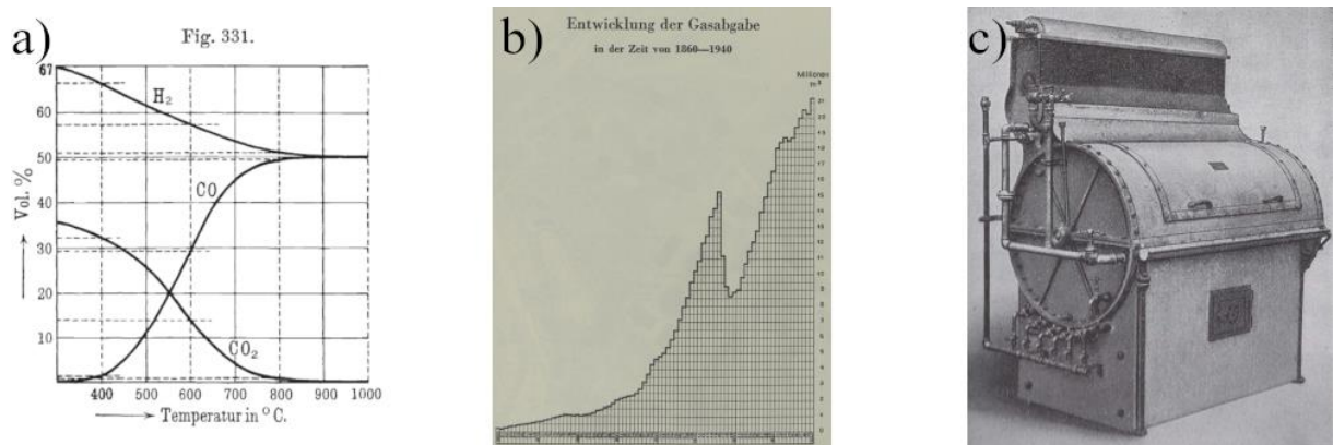
Figure 2: (a) H_2:CO ratio in relation to reactor temperature for water gas [7]. (b) Annual gas production from 1860 to 1940 in Mm^3 of the gasworks Bern. The sharp decrease around 1919 was caused by coal shortages during WWI [4]. (c) Washing machine with gas heating [5].
