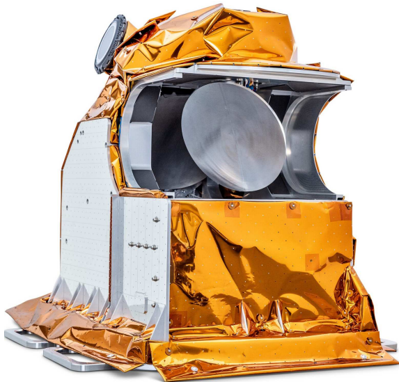
FIGURE 1. Picture of AWS Protoflight model. Flight direction is upwards in the image. Nadir view is out of page. Scan direction from right to left. Courtesy of AAC Omnisys.
