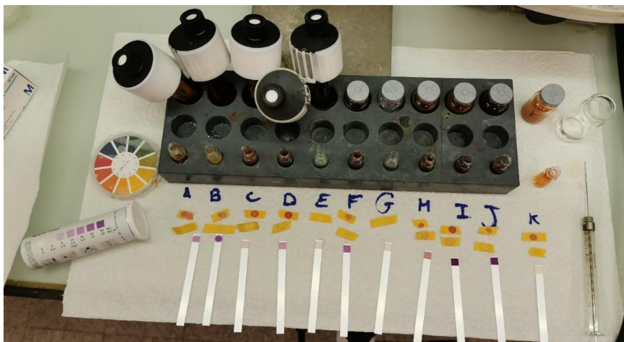
Figure S10. Results of nitrite tests of reaction medias with colorimetric test strips (colorimetric, 2-80 mg/L ( \text{NO}_2^- ), MQuant, SKU: 1100070002). The results of nitrite tests are represented below in Table S9.
