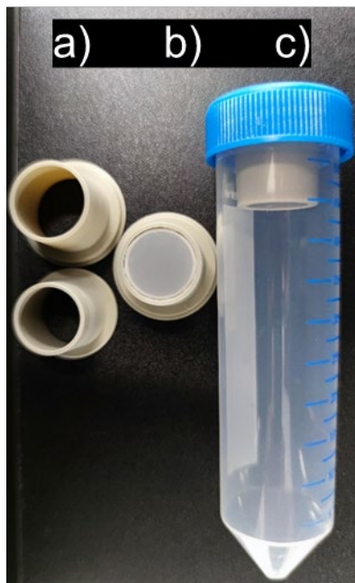
Figure S1: Dialysis device for drug release experiments a) disassembled without a membrane, b) assembled with a 100 nm polycarbonate membrane and c) inside a 50 mL conical tube.
