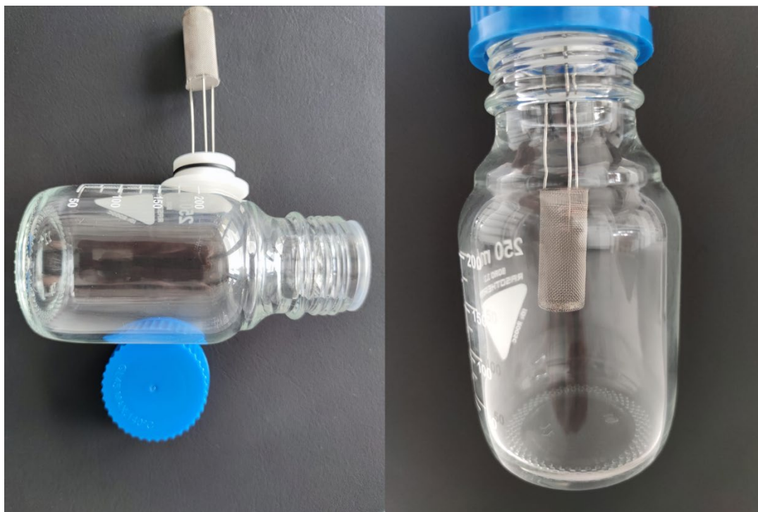
Figure 22: Release study setup for bulk RAPA-LMPs.
