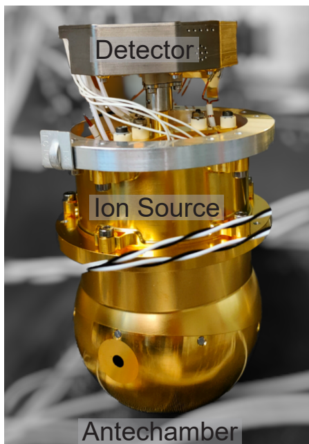
FIGURE 6.4: Ion source connected directly to the detector.
