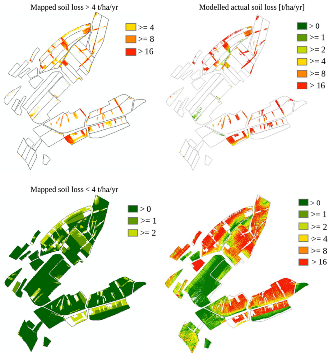
Fig. 5. Mapped soil loss in the soil loss categories >4 t/ha/yr (top left) in the Frienisberg region and modelled soil loss for the corresponding areas (top right). Mapped soil loss in the soil loss categories <4 t/ha/year (bottom left) and modelled soil loss for the corresponding areas (bottom right).
