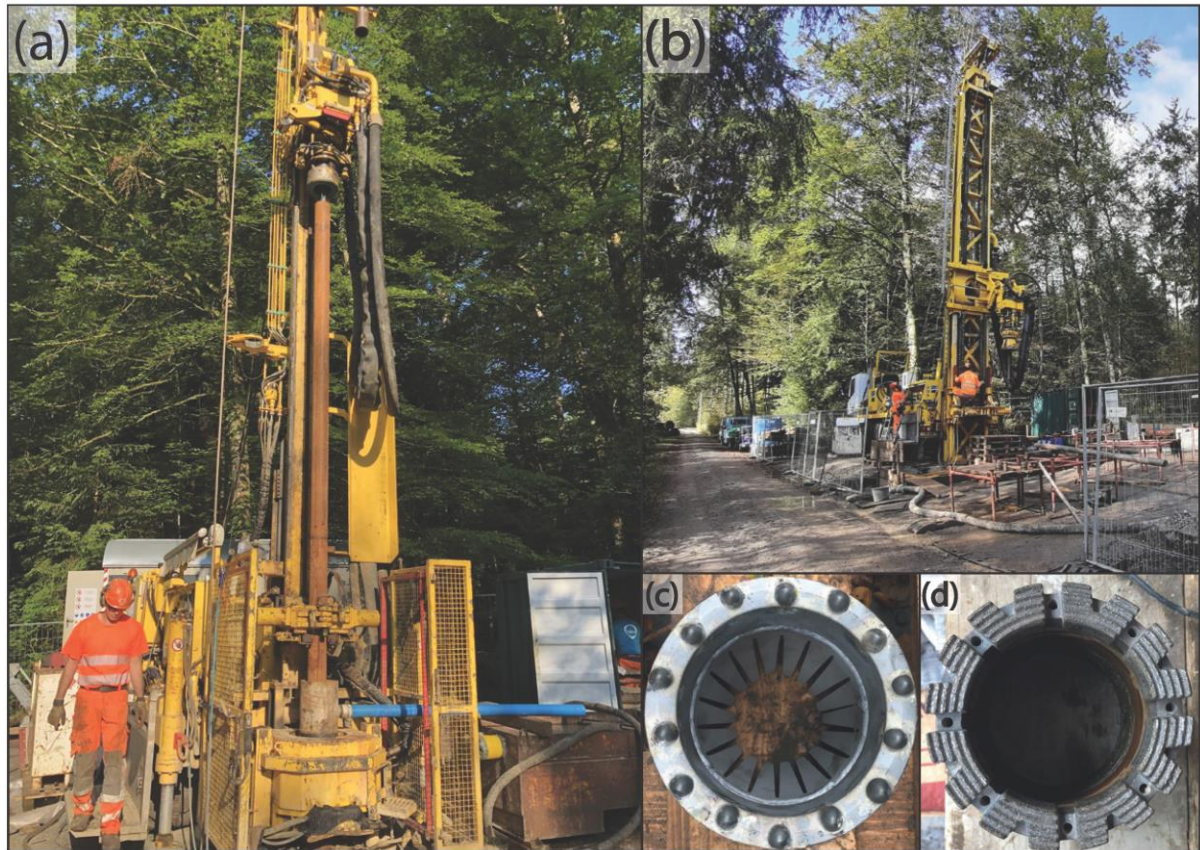
Figure 2: (a) Drill rig used from 0 to 228 mtd (meters total depth); (b) drill rig used from 228 to 252 mtd; (c) drill bit used during percussion-hammer coring to a depth of 57 mtd; and (d) diamond and hard-metal drill bit used during rotary drilling below 57 mtd (photos by Sebastian Schaller).
