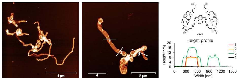
Figure 7.66: AFM images of the self-assembled CPC3 with cross section on an APTES-modified mica sheet. Conditions: 3 \mu\text{M} oligomer, 10 mM sodium phosphate buffer, 10 mM NaCl and 15% EtOH.
