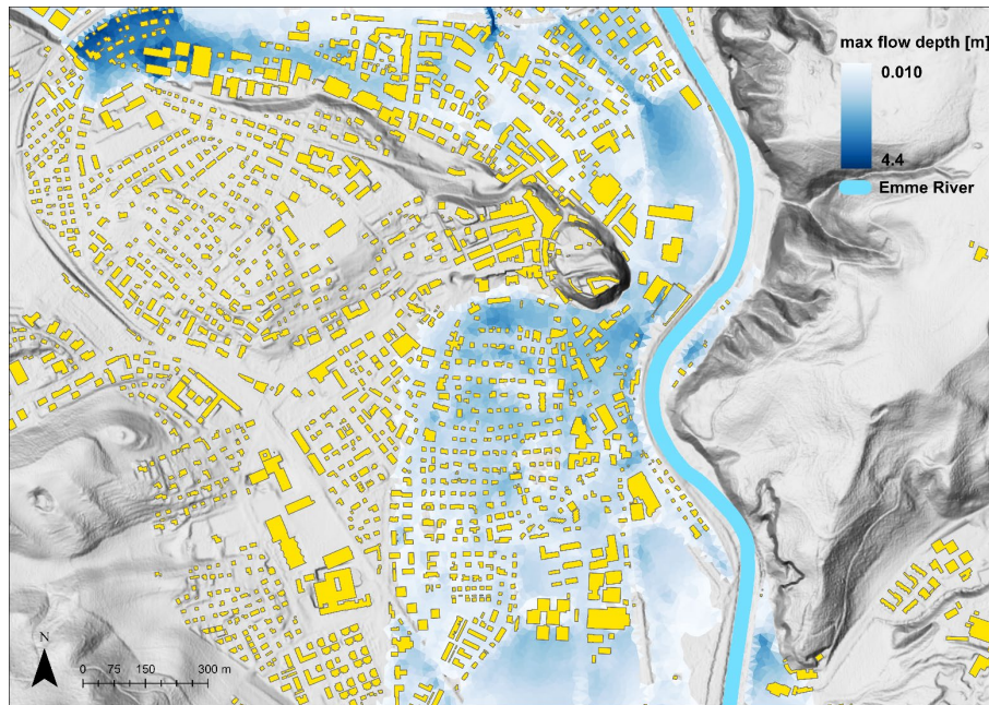
Figure 4-7. Map of a flood simulation with a peak discharge of 1200 m 3 /s. Light blue symbolize low flow depths and dark blue symbolize high flow depths. The upstream boundary is in the South, water flows from South to North. Building footprints are visualized in yellow 58 . Background: Digital Terrain model, swissALTI3D66.
