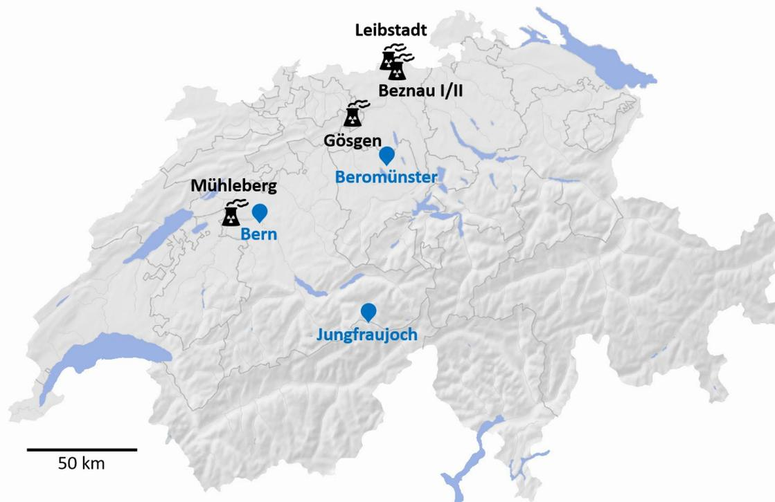
Figure 3.1 Geographical map of Switzerland, with the sampling sites (in blue) and the five nuclear power plants (in black). Gösgen and Beznau I/II hold a PWR (emitting mostly  $^{14}\text{CH}_4$ ), whereas Mühleberg and Leibstadt hold a BWR (emitting mostly  $^{14}\text{CO}_2$ ).
