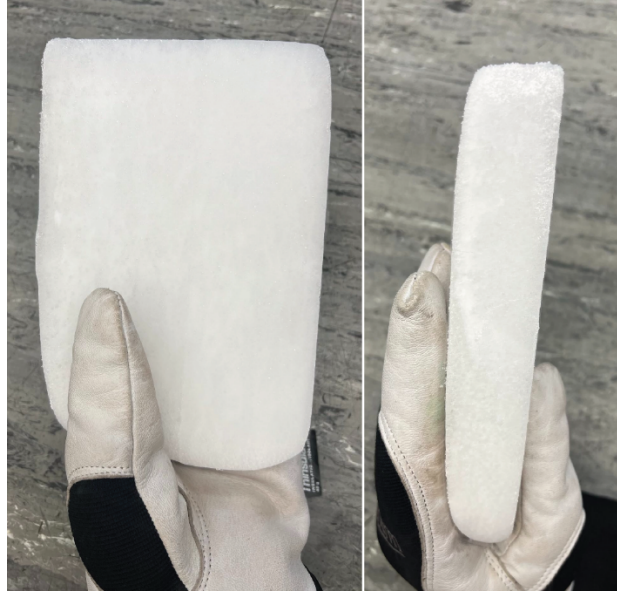
Figure 3.12: CO 2 plates produced by Carbagas (item n°I5801) and used as analogue in the self-cleaning simulations (see section 5.1). The pristine dimensions are 250x125x30mm.
