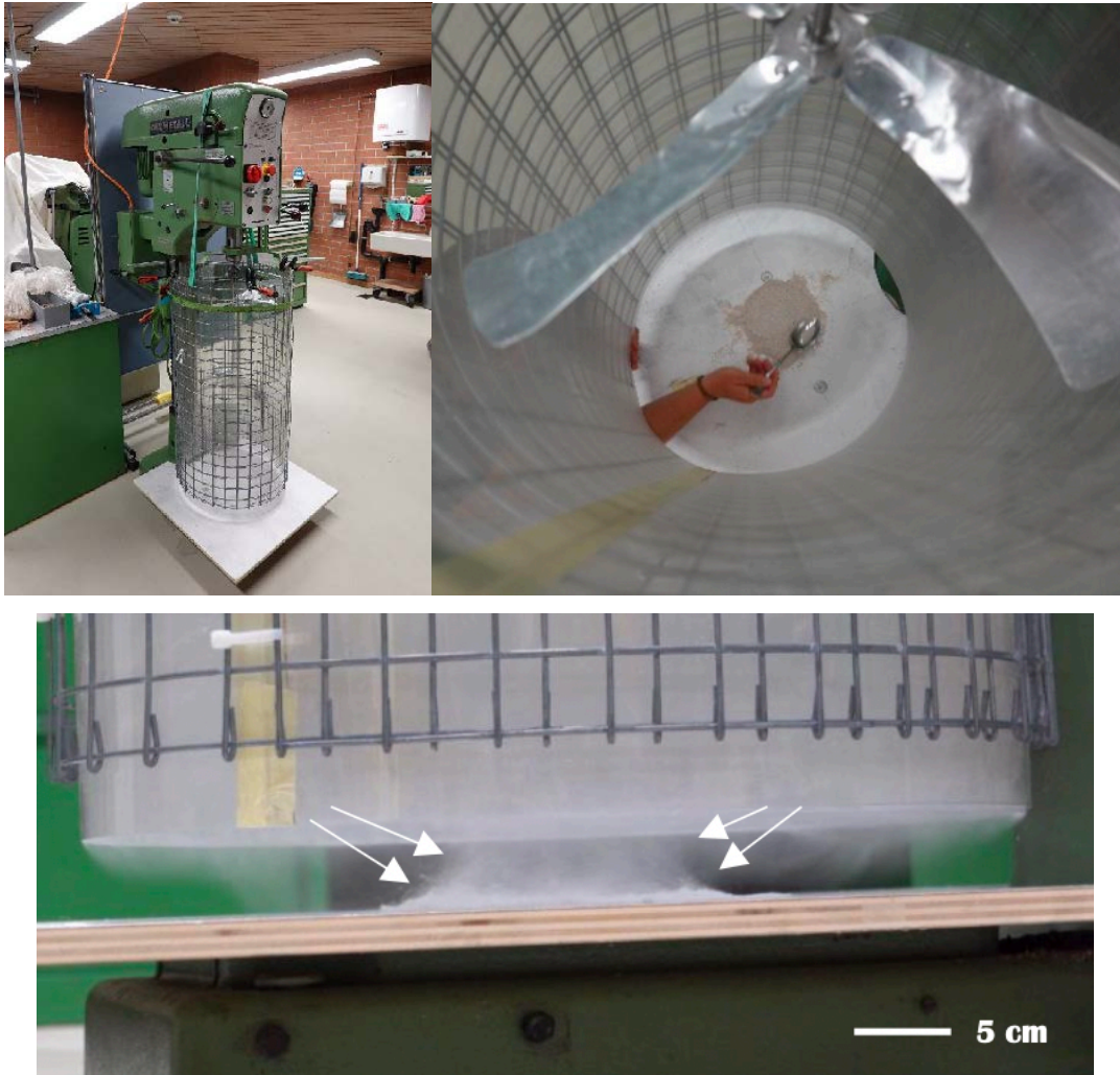
Figure E.1: (Top row) Images of the full setup (left) and view from the rotating blades (right). (Bottom) Formation of a vortex using microgrit aluminium powder. Extracted from Michelle's report.
