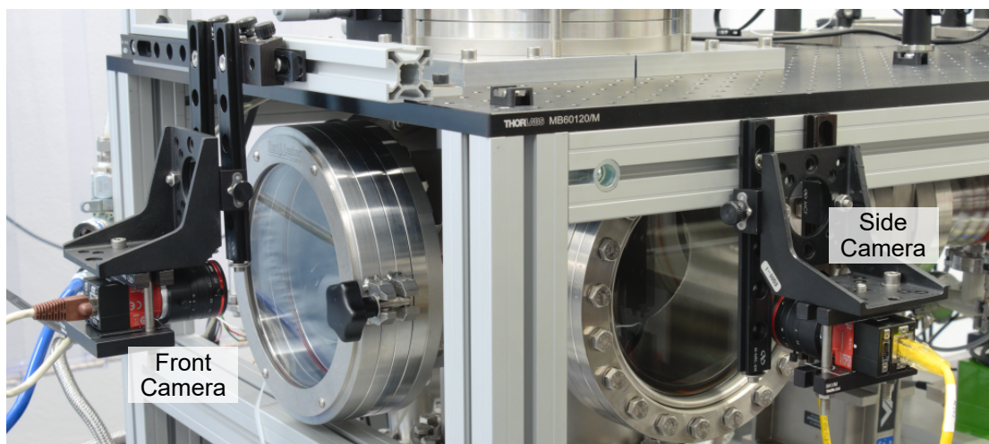
Figure 2.13: ORIGIN chamber with two orthogonal viewports. The cameras of the observation system are mounted to the setup using dovetail rails for alignment purposes and point towards the ablation region.
