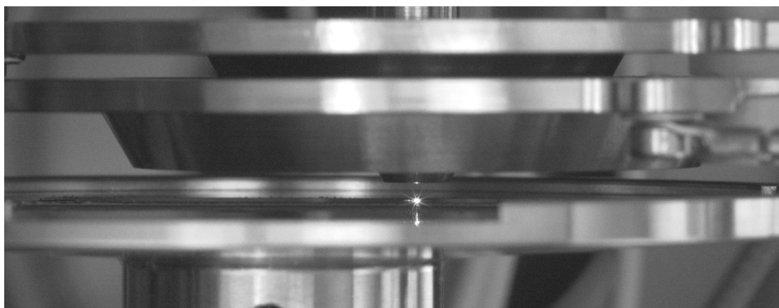
Figure 2.14: Ablation region as imaged by the front camera. The location of the laser beam in relation to the mass analyser entrance and the sample is clearly visible.
