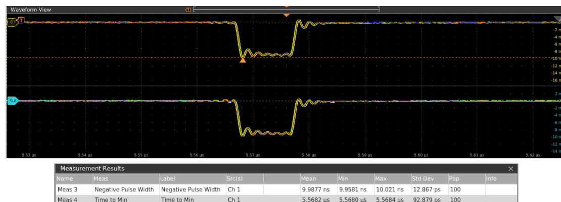
Figure 4.16: Oscilloscope measurements of the LG and HG signals using a Tektronix MSO64B. The oscilloscope was configured to trigger on the generated “Laser Sync” signal, thus being able to measure the jitter between the two signals.
