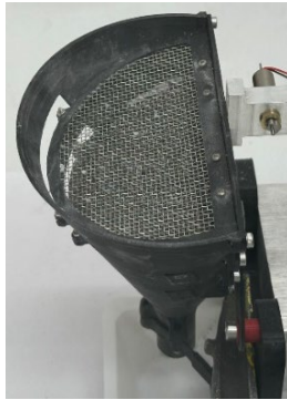
Figure 9: 3D printed funnel with 63^\circ wall angle used to test and validate the sieving performance.
