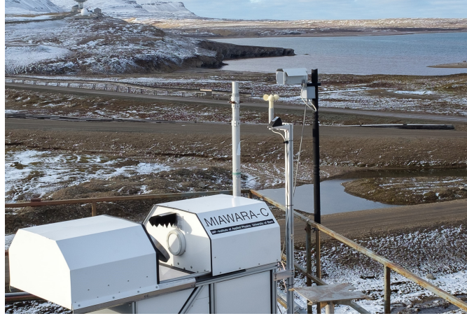
Figure 2.4 The ground-based microwave radiometer MIAWARA-C at Ny-Ålesund.
