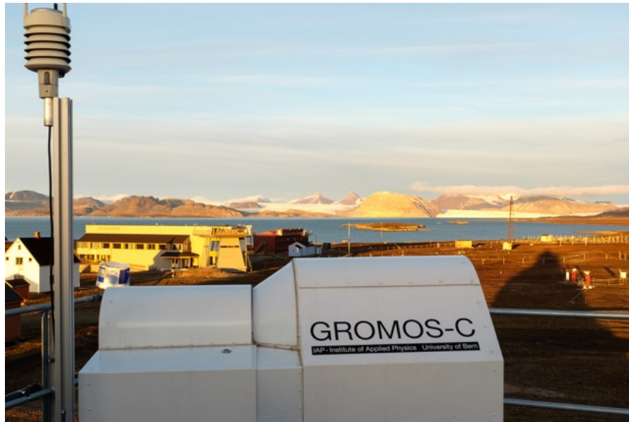
Figure 2.2 The ground-based microwave radiometer GROMOS-C at Ny-Ålesund.
