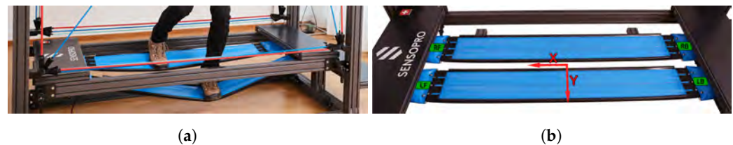
Figure 1. The tapes of the Sensopro Luna during a sideways exercise (a) and at rest (b), with green markings indicating the IMU positions. Blue plastic covers are screwed onto the tape, hiding the springs. The anchor points are below the black platforms at the front and back.
