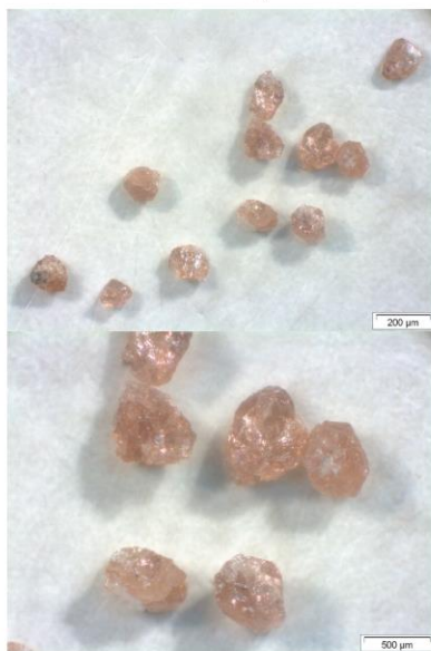
Mafic fels - Z18TB15 diameter: 250 - 500\mu\text{m}
