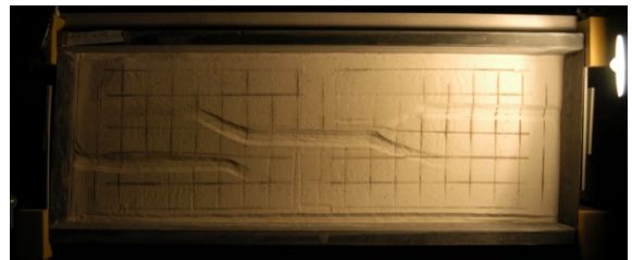
-30° oblique extension models. Angle \phi = 60^\circ , and 30^\circ . Rerun of EXP509, since we had strange linkage (parallel to extension direction), which happened again in this model (for the \phi = 30^\circ model). No coherent results, the rift even propagated even towards the other rift.
