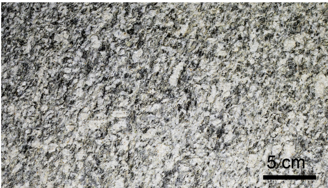
Figure 2.11. Picture from the GTS showing the typical appearance of Grimsel Granodiorite. Photograph taken at L510.
