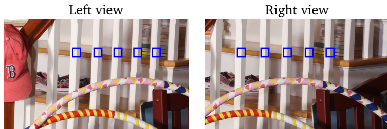
Figure 1.2: Visualization of the disparity ambiguity in matching pixels from the left view to the pixels in the right view (Middlebury Stereo Dataset [SHK + 14]). Each of the blue boxes in the left view could be matched with all other boxes in the right view.
