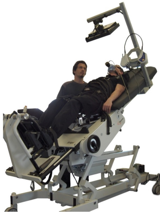
Figure 1. A modified robotics-assisted tilt table (RATT) with force sensors under the thigh cuffs, visual feedback system and breath-by-breath cardiopulmonary monitoring system.
