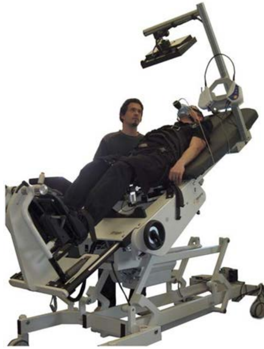
Figure 2. The augmented robotics-assisted tilt table (RATT) system with force sensors under the thigh cuffs, visual feedback system and breath-by-breath cardiopulmonary monitoring system.
