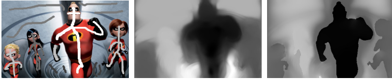
Figure 4.7: Input image with scribbles (left), continuous disparity map (middle) and discontinuous disparity (right). Wang et al. [91].
