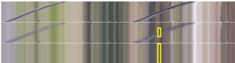
Figure 5.12: On top the input EPI consisting of 36 images. The one in the middle we blurred vertically with a 7 rows wide Gaussian filter ( \sigma = 2.5 , yellow box). The bottom one is filtered with a box filter, considering all rows (magenta box), what we do for infinite apertures.
