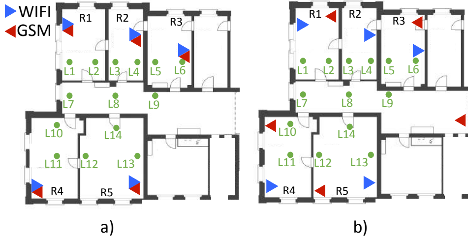
Figure 5.7: a) colocated antennas setup. b) distributed antennas setup
